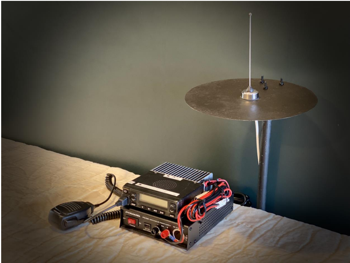
Typical 15-40 Watt Base Station with One Type of Outdoor Antenna
