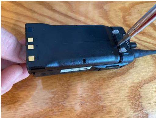
In rare cases, the battery may get stuck. You can use a screw driver to release it. Remove the battery in the same way as described above, but insert the screw driver in the space between the battery and radio housing at the top of the battery. Twist the screw driver and the battery will slide out easily.
