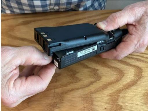
To remove the battery from the radio: Turn the radio over. Slide the catch on the bottom of the radio with one thumb while you press against the top of the battery with the other. The battery will slide out of its holder.
