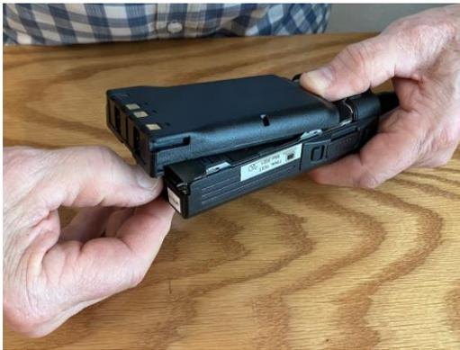
To remove the battery from the radio: Turn the radio over. Slide the catch on the bottom of the radio with one thumb while you press against the top of the battery with the other. The battery will slide out of its holder.
